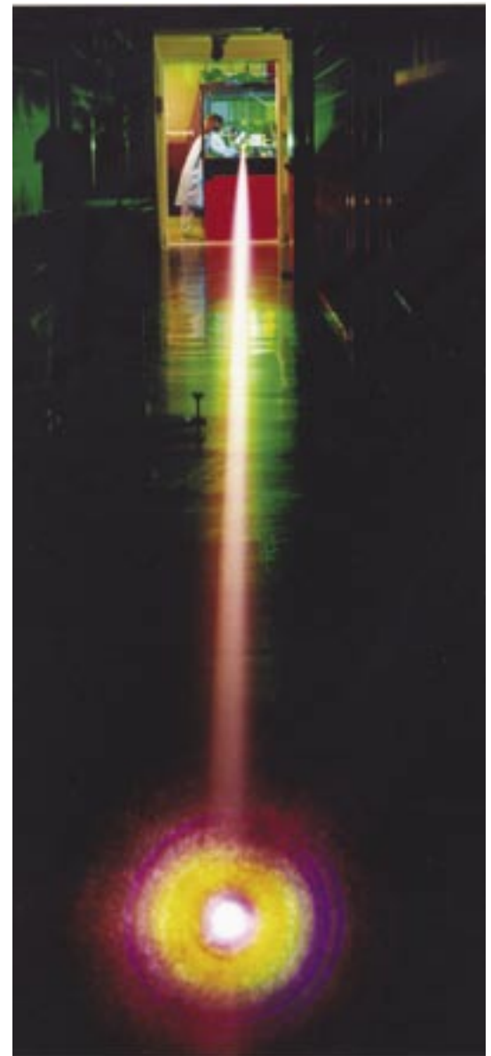
Ultrafast, Chirped Pulse Amplification (CPA) laser. The long filament is a result of channeling. [Photograph by William Pelletier, Photo Services, Inc.]
